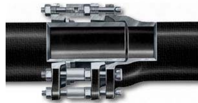
Figure 2.5 – Mechanical Coupling Joint 4
