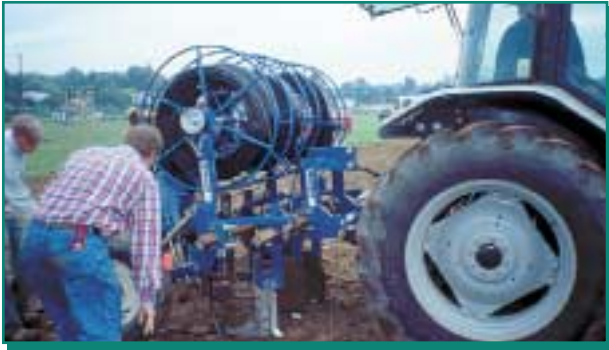
8-9-10. Drip tubing being installed
