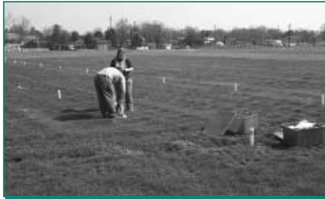
▲ 16. Sampling lysimeters over turf areas.
