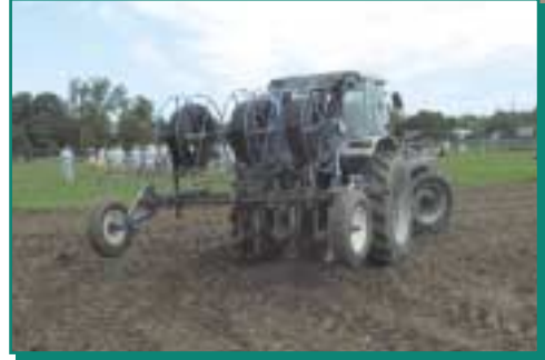
7. The drip tubing is then installed at 9 to 11 inches beneath the surface.
