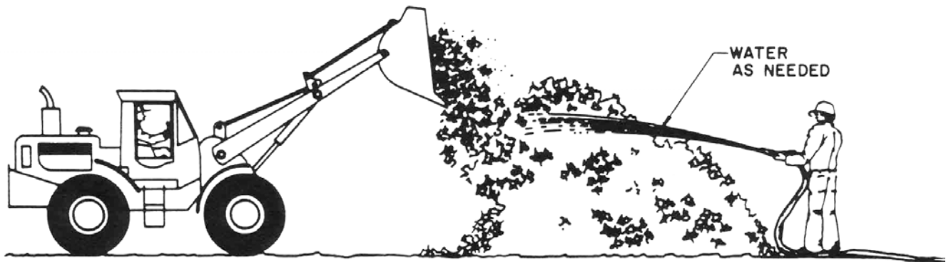
STEP 5. TURNING PILE IN PLACE
