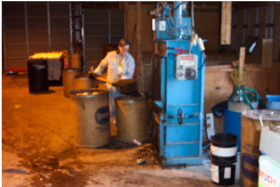
Figure 2 Manual Loading of Material into a Baler
