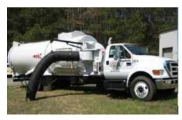
Impac's compaction bodies offer a perfect solution for those seeking the most from their waste transportation systems. The Impac is a side-loading compaction system perfect for curbside loading. And being fully automated for the one-man, in-cab operation with its high compaction storage area, it helps to keep overhead down allowing for more time spent picking up and less time dumping.
