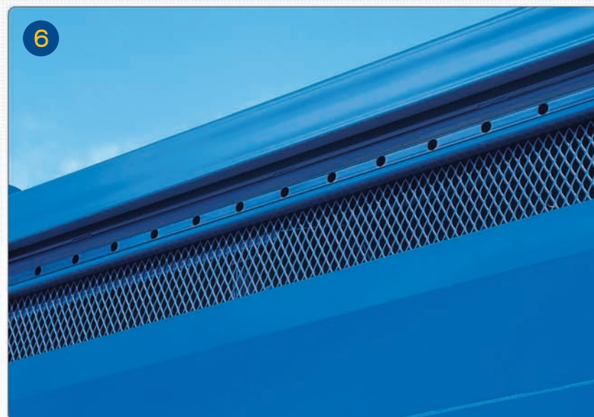
6. Steel mesh along top of body offers visual check on material level for easy on-the-route adjustability, and can be used to monitor the position of the Maximizer™ panel. Both interior panels and loading bucket separators adjustable at 6" (152 mm) intervals.
