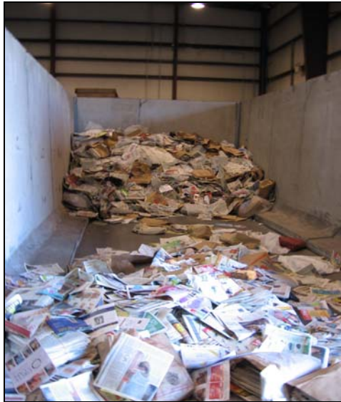
Figure 2-5 Sorted Newspaper Storage Bunker
