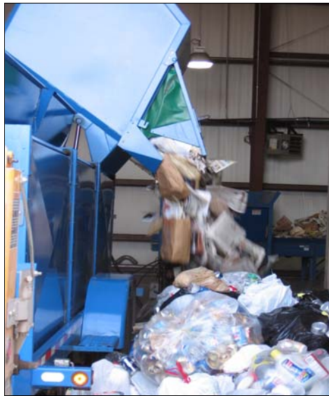
Figure 2-2 Municipal Haul-All Container Tipping at Recycling Center
