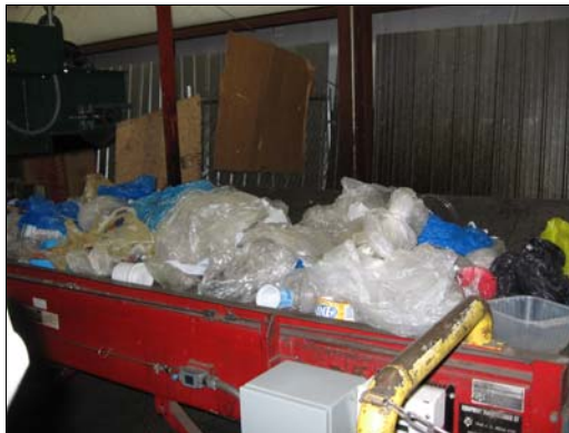
Figure 2-7 Residue at End of Sort Conveyor
