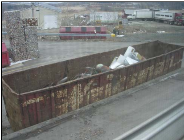
Figure 2-6 Scrap Metal Roll-Off Container
