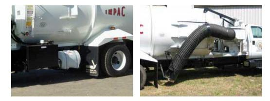
The IMPAC compactors are manufactured to strict A.S.M.E. code welding procedures in a variety of capacities from 20 to 33 cubic yards. You also have a choice of right or left hand side pickup styles with many standard features that are considered optional on other vehicles. The IMPAC is quick, having cycle times less than 30 seconds when handling steel or plastic containers, from 24" to 55" in diameter.
