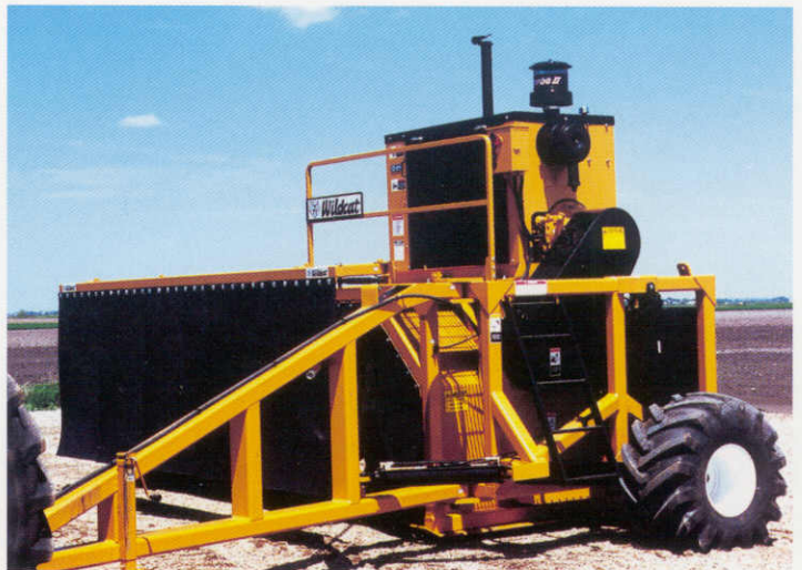
Hitch folds hydraulically for ease of transport.
