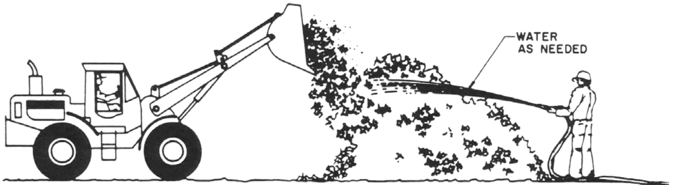
STEP 5. TURNING PILE IN PLACE
