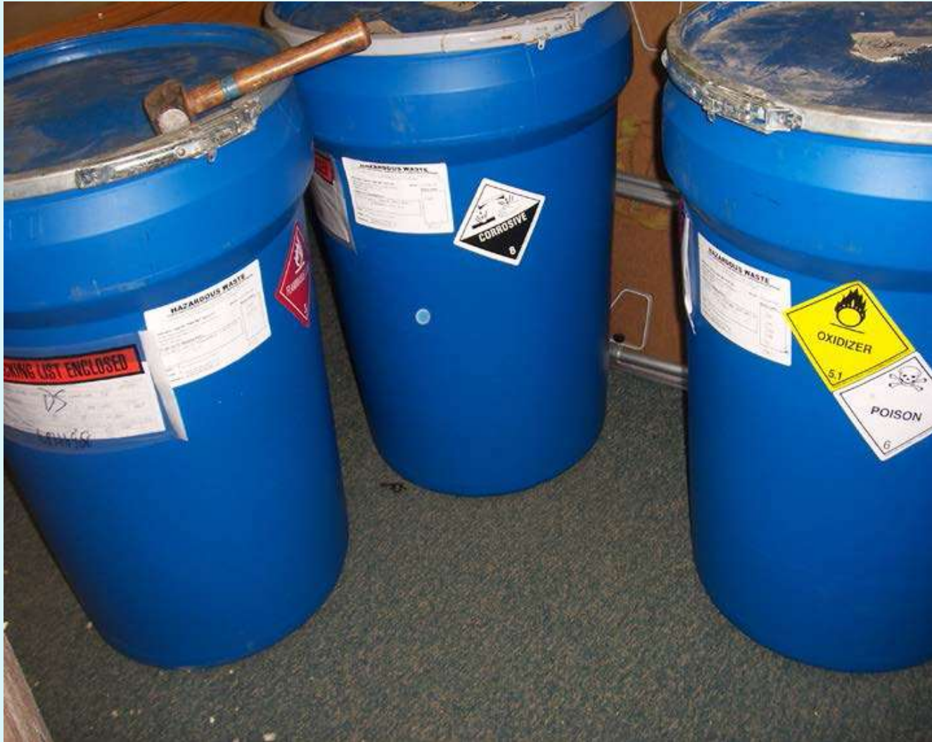
Transportation containers with Hazardous Materials warning labels
