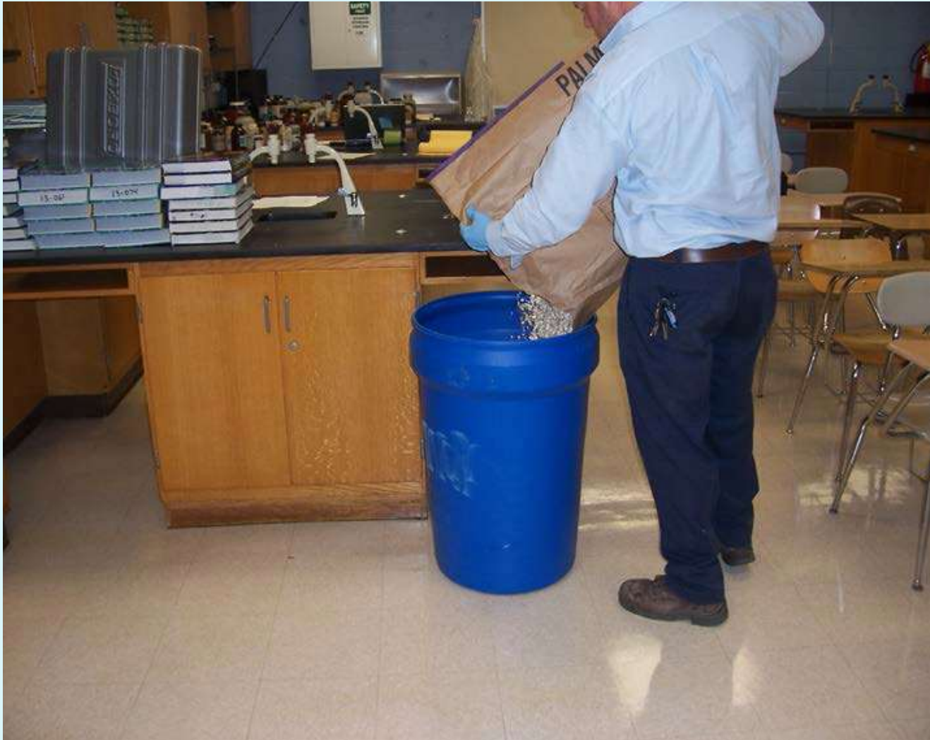
Absorbent material being added to transportation container
