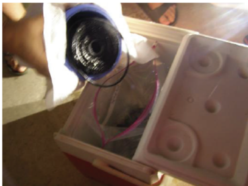
Removed sediment filter 9-27--25 @ 9:41
