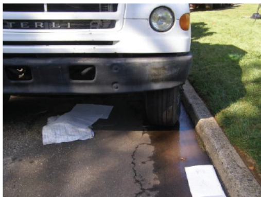
Absorbent pads under drill vehicle and sheen on water along curb in front of [redacted]
