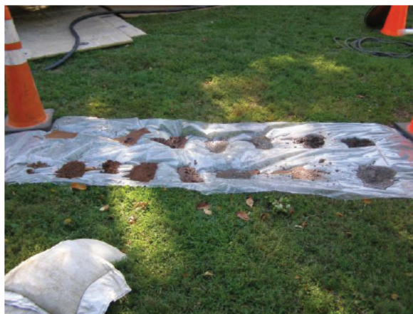
Soil samples from every 5 feet while installing MW-11D 9-8-25
