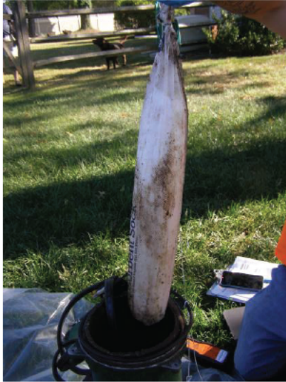
Absorbent sock removed from potable well at [REDACTED] 9-2-25 @ 9:15
