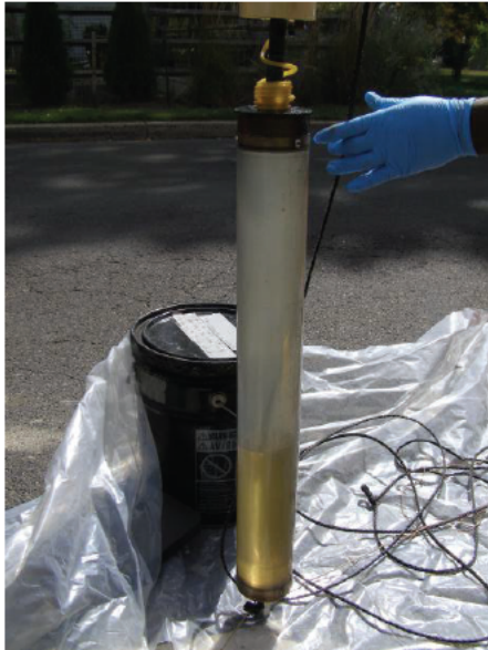
LNAPL in the skimmer from recovery well RW-2 9-2-25 @ 10:45
