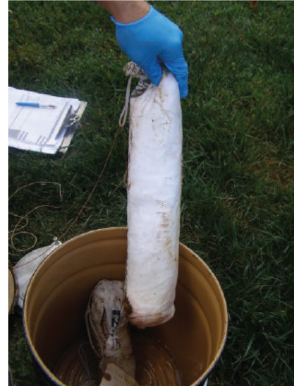
Absorbent sock removed from the potable well at [REDACTED] 9-2-25 @ 9:38
