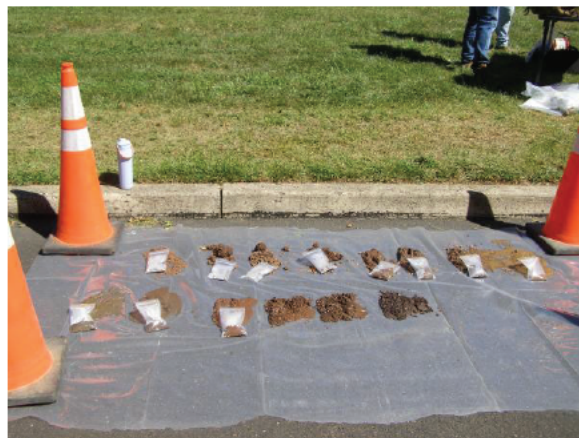
Soil samples collected between 10 and 75 feet bgs in well hole 8-26-25 @ 11:15 am
