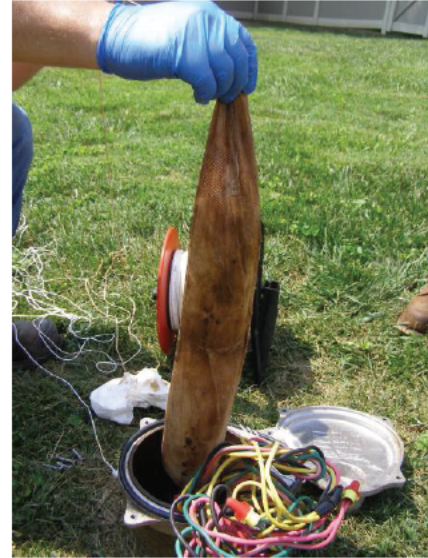
Absorbent sock in potable well at [REDACTED] 8-7-25 @ 11:33am
