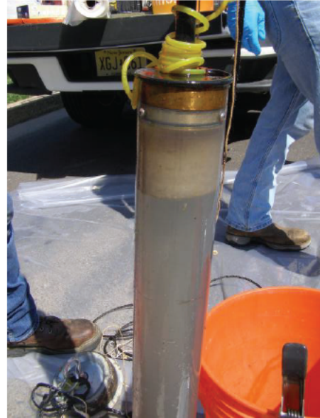
LNAPL in removed skimmer from RQ-2 8-11-25 @ 10:49am
