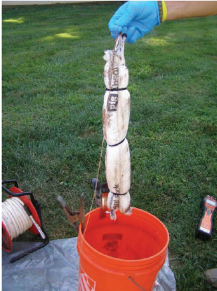
Three absorbent socks in potable well at [REDACTED] 8-11-25 @ 10:11am
