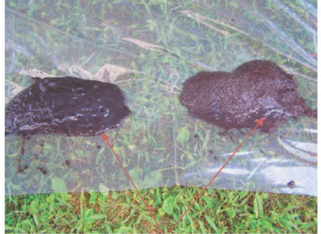
Close up of the coal shale present in the soil samples between 70 and 75 feet bgs. 7-31-25
