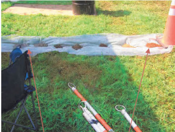
Soil samples from the installation of MW-1S 5' feet below ground surface 45' below ground surface 7-31-25
