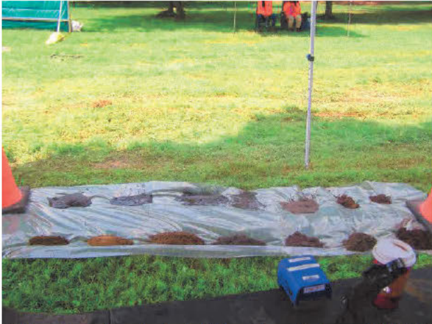
Drill cuttings from the installation of monitoring well MW-2D 7-31-25
