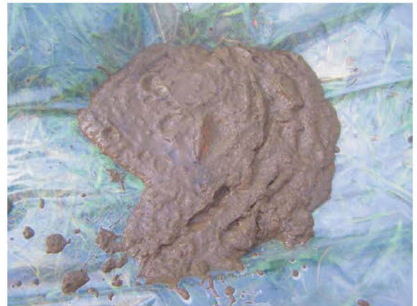
Coal shale present in soil sample from MW-1S at a depth of 45 feet bgs. 7-31-25
