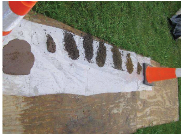
Photo 2: Staging of soil cuttings from 5-foot intervals
