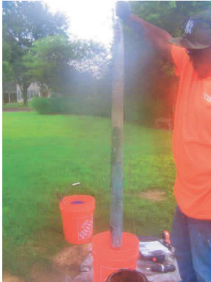
Absorbent sock pulled from potable well at [REDACTED] 7-7-25 @ 9:18
