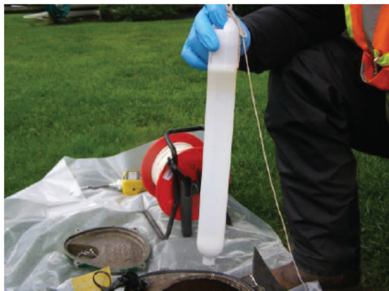
LNAPL in potable well at [REDACTED] 5-22-25 @ 9:31
