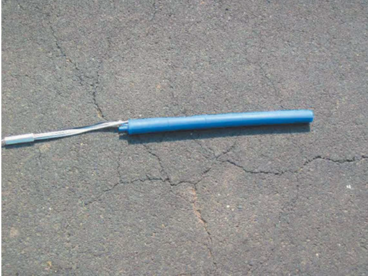
Submersible pump used to purge RW-2 and RW-3.
