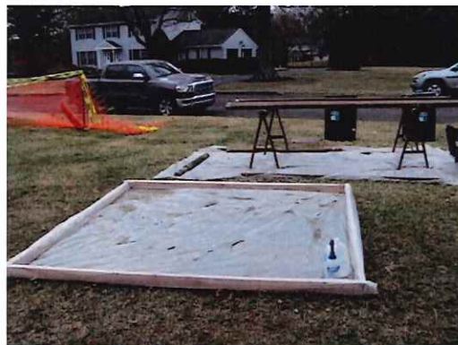
Decon Station for Packer Test at 108 Spencer Road 3-14-25
