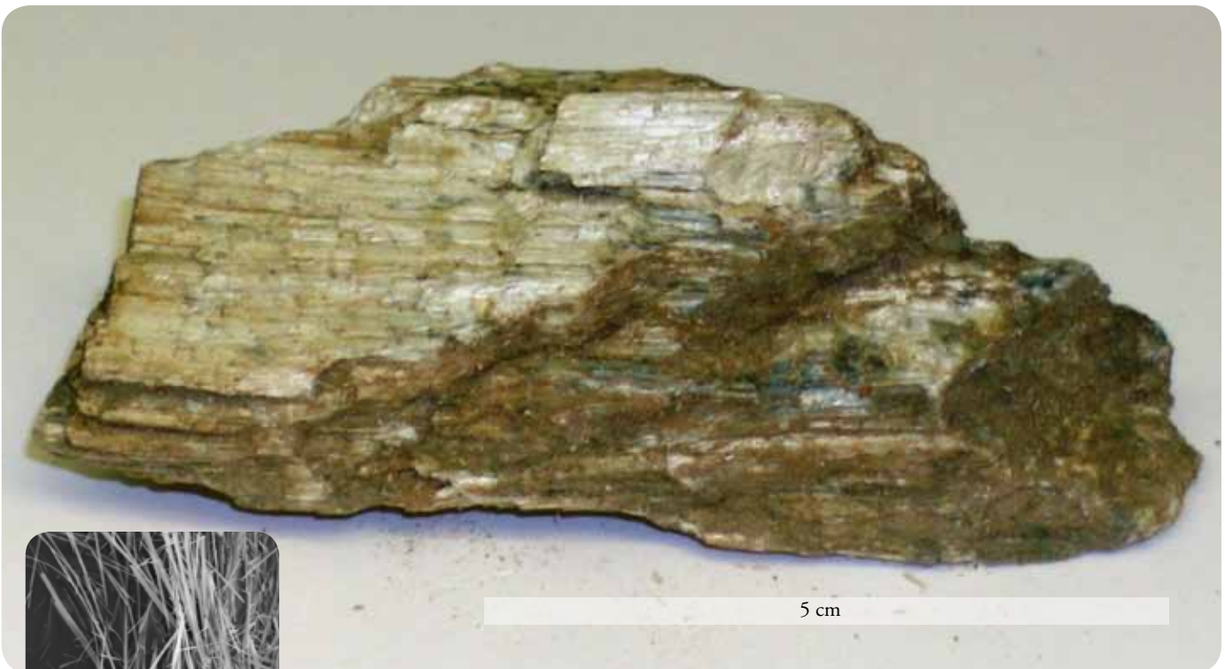
Photo of asbestiform tremolite, El Dorado County, California seen in hand sample (above) and scanning electron micrograph (left), courtesy of US Geological Survey, Denver Microbeam Laboratory.
