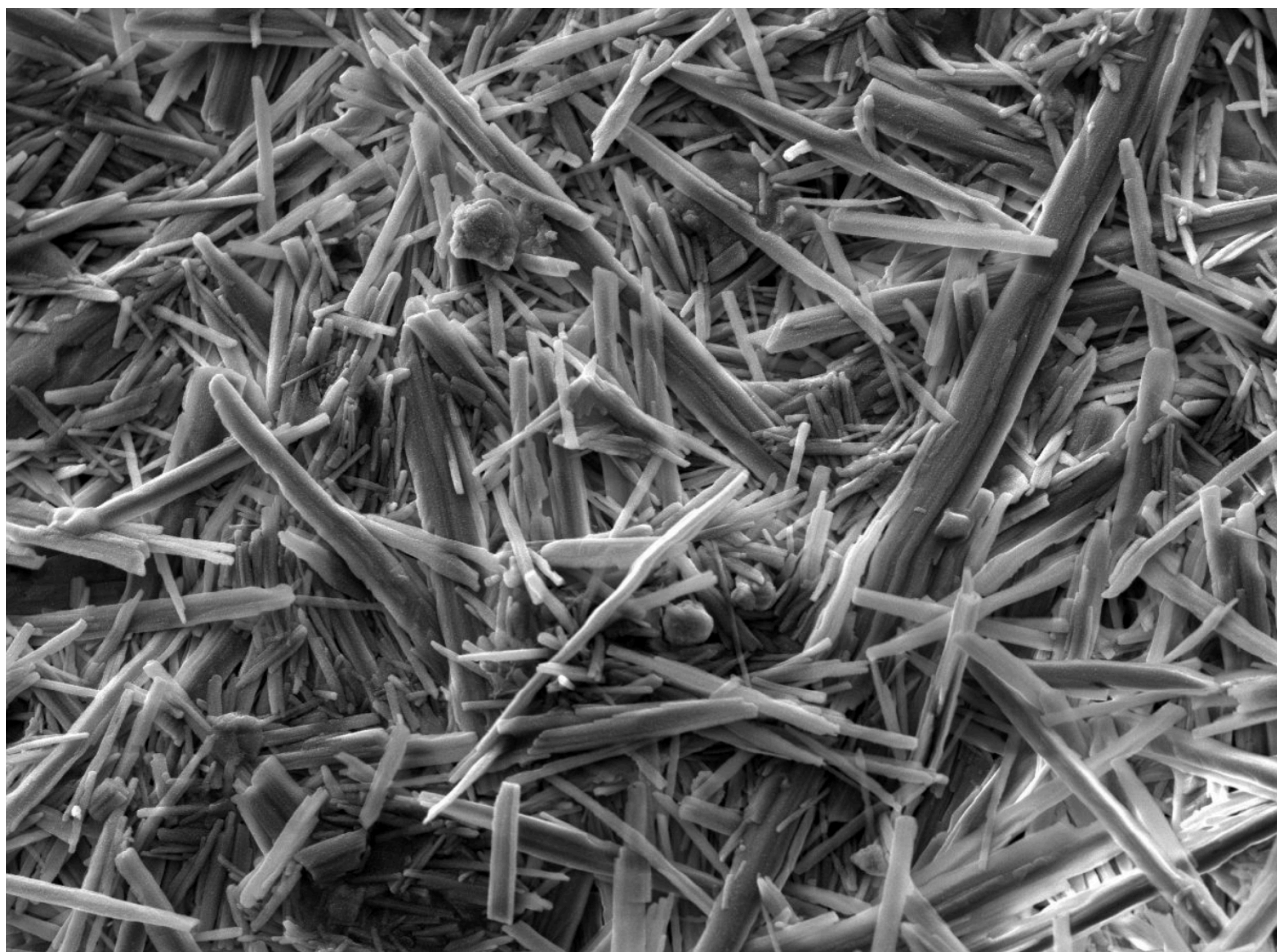
Figure 1: Scanning Electron Microscopy (SEM) photomicrograph of tremolite asbestos rock fragment collected within the Franciscan Complex in the San Francisco Bay Area region of California. Note the numerous fibers with rounded, pointed and cleft ends, non-parallel sides, and non-perpendicular ends, all of which would be eliminated using EMSL's and RJLG's differential counting criteria.
