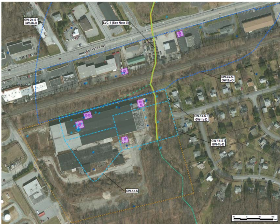
Figure 2: Snapshot of part of FS Figure 17 showing functional areas as identified for remediation of organic contaminants. There are three onsite areas, GW-1a, b, and c, and two offsite areas, GW-2a and b, and LVC and tributary east of the site. The purple areas are DNAPL FAs. Each groundwater FA has a shallow (overburden and shallow bedrock) and deep (intermediate and deep bedrock) layer. GW-1d is an area of inorganic contaminants that includes most of the three onsite areas (not shown).
