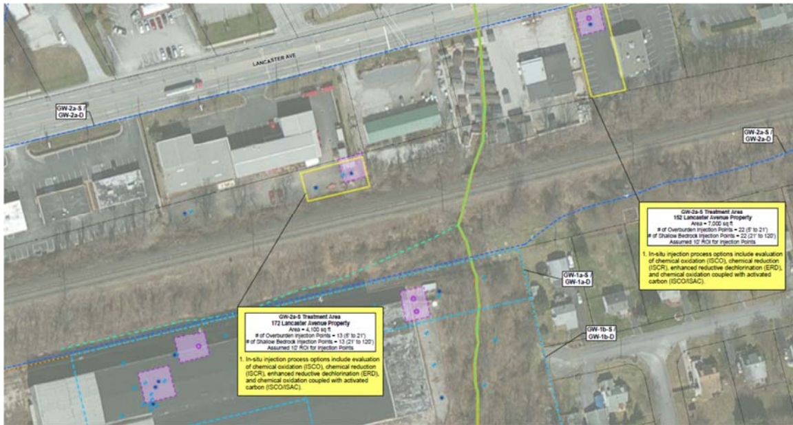
Figure 4: Snapshot of FS Figure 20b showing the areas for offsite injection in alternatives 3 through 6 in FS GW-2a-S. The outlined injection sites would include injection points located on 10 ft radii of influence in the overburden and shallow bedrock layers.
