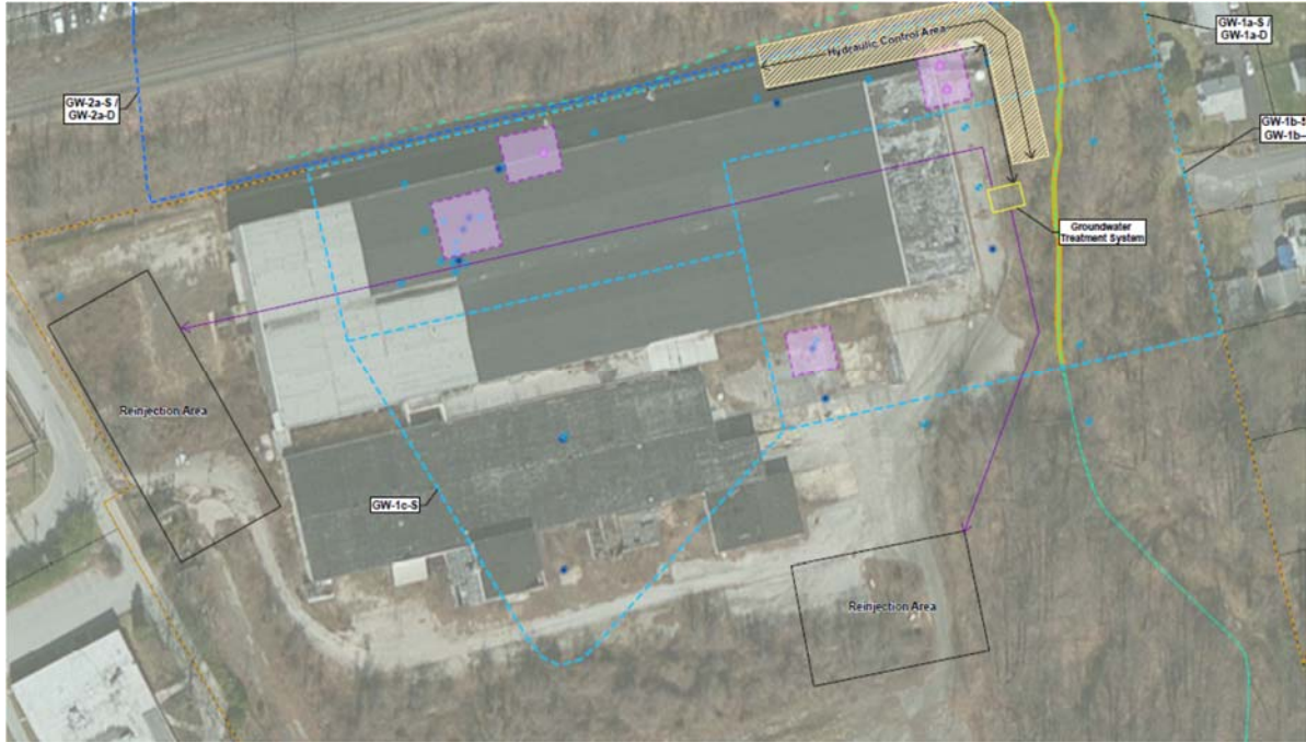
Figure 6: Snapshot from FS Figure 19a showing location of extraction and reinjection zones for alternative 7.
