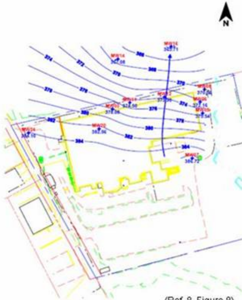
Figure 3 Shallow/Overburden Monitoring Wells BISHOP TUBE SITE WATER TABLE CONTOUR MAP (OVERBRDEN WELLS) MARCH 31, 2003
