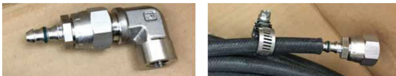
Figure 3.14 – DEF Line Connection to the Injector Lance
