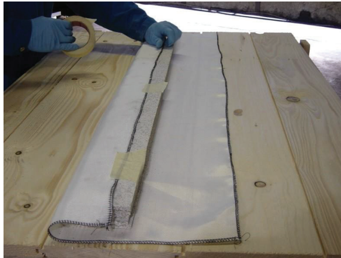
Figure 12: Assembling an Expansion Mat Bundle
