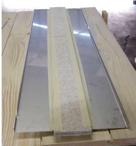
Figure 15: Securing Expansion Mat on Door Tray
