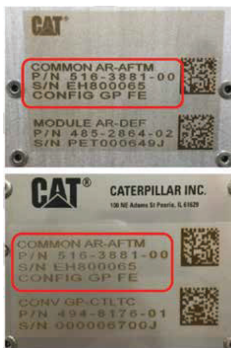
Figure 2.4 – Dosing Cabinet and CEM Common Arrangement Identification Plate Examples
