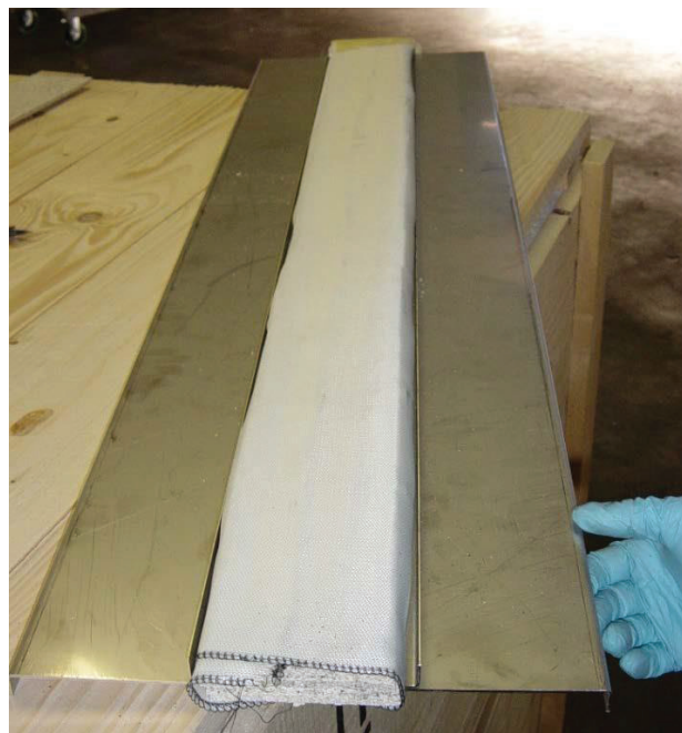
Figure 13: Example of an Expansion Mat Bundle Installed in a Top Tray
