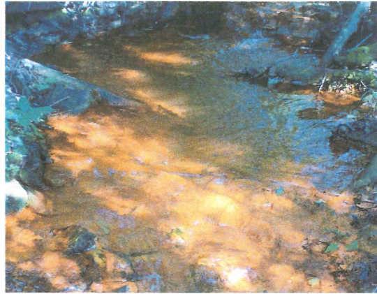
Monitoring Point 2. Saltlick Run at Pottersdale Road. Heavily impacted by acid mine drainage from abandoned mine lands showing dense iron precipitation on stream bed. No aquatic life present.
