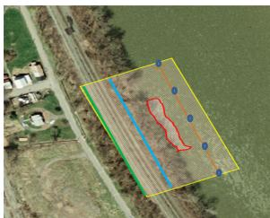
The five blue dots represent five depth measurements to be averaged along midpoint between shoreline and outer boundary of AA.
