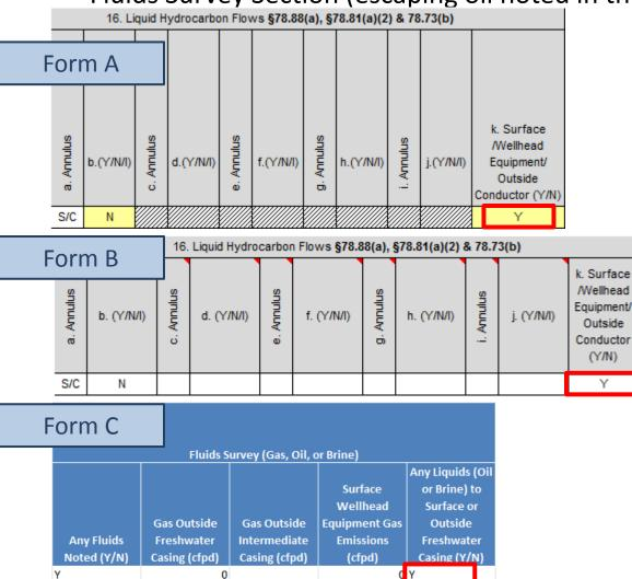
In this case, an oil leak resulting in the release of oil to the ground surface was noted in association with the surface wellhead equipment. No leaking brine or gas was noted. Because an oil leak is noted, a "Y" must be placed in the field labeled "Any Fluids Noted" in Form C.
