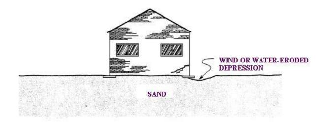
Cracking of Masonry Wall Due To Foundation Undermining by Surface Erosion
