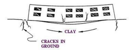
Shrinkage of Clay Under Center of Building
