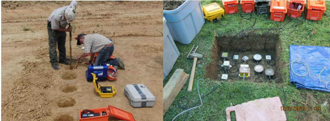
Figure 1. Linear geophone deployment (left); Cluster geophone deployment (right).
