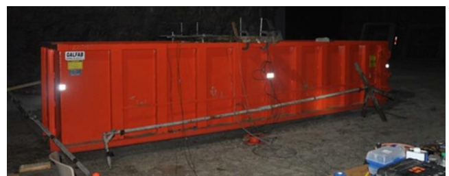
Above Figure: Sand Tank Setup to measure excess pore pressure
