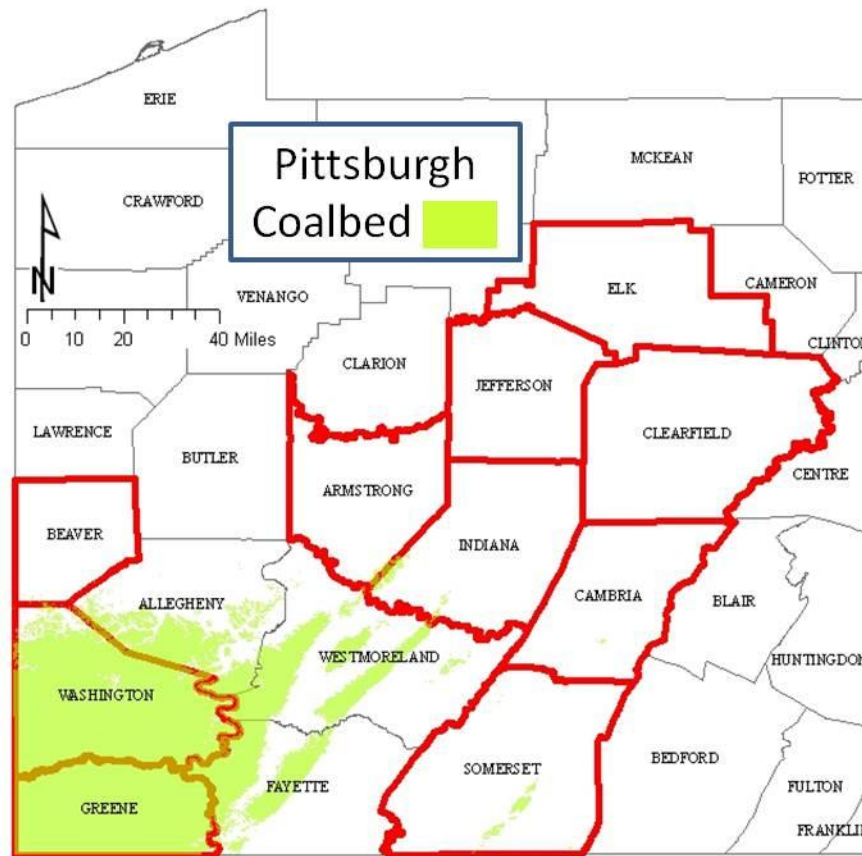
Figure III-6 - Areas underlain by the Pittsburgh Coalbed. Note - While current mining in the Pittsburgh Coalbed is largely limited to Greene and Washington Counties, drift and shaft mining have occurred in Allegheny, Armstrong, Fayette, Indiana, Somerset and Westmoreland Counties over the last 100 years.
