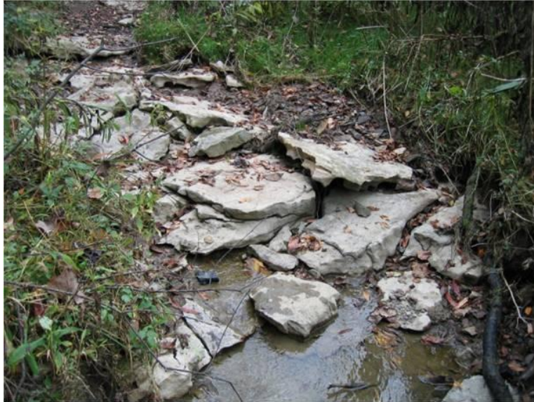
Figure D-10 – Compression ruptures observed by PA DEP in the F8 panel during a post-mining survey (Photograph from PA DEP files).
