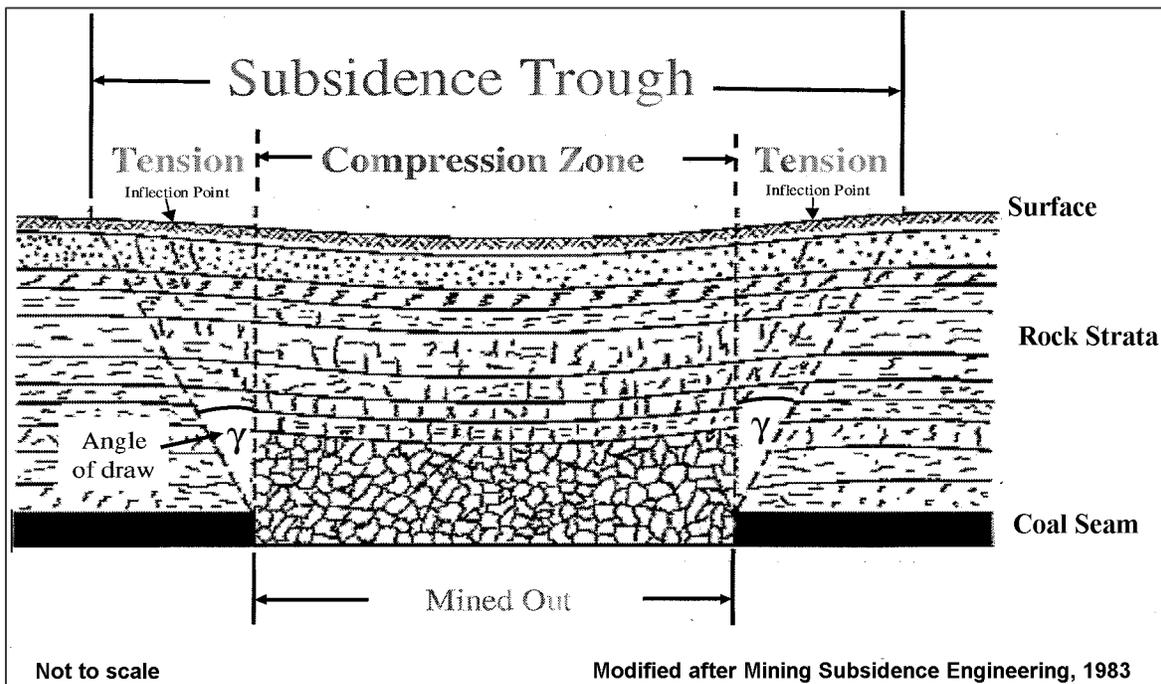
Ground movements within a subsidence trough have both vertical and horizontal components. Downward vertical movement usually occurs at all areas within the trough. The vertical movement is usually greatest at the center, and it progressively decreases at points along the trough profile until the limit of the affected surface area is reached. The Department's investigators have also observed instances where slight "heave" or upward movement has occurred.
