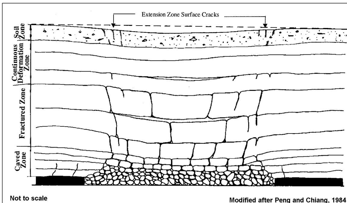
Various researchers use different vertical distances to mark the transition points. However, the numerous independent studies paint a similar composite picture of the vertical fracture profile above longwall panels.
