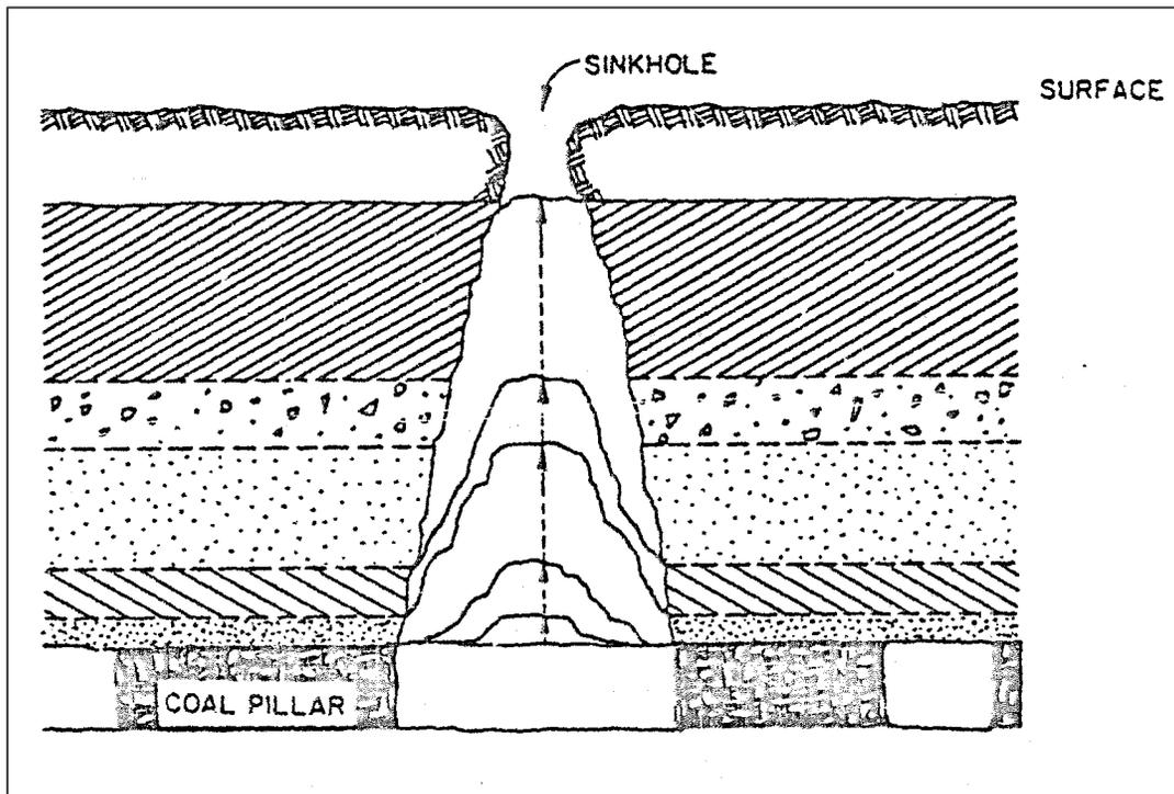
The majority of sinkholes usually develop where the amount of cover (vertical distance between the coal seam and the surface) is less than 50 feet. This type of subsidence is generally localized in extent, affecting a relatively small area on the overlying surface. However, structures and surface features affected by sinkhole subsidence tend to experience extensive and costly damages, sometimes in a dramatic fashion. Sinkhole subsidence has been responsible for
