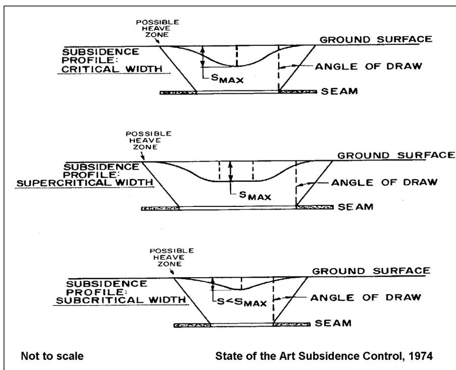
As the face advances to areas below and beyond the structure or feature, the ground surface may then be in compression since it is now located near the center of the existing subsidence basin. Cracks and separations, which previously appeared, may now close only to give way to new cracks, and perhaps buckling of foundation walls. The structure or feature may also return to its previous state of level and plumb relative to the longitudinal axis of the panel.
