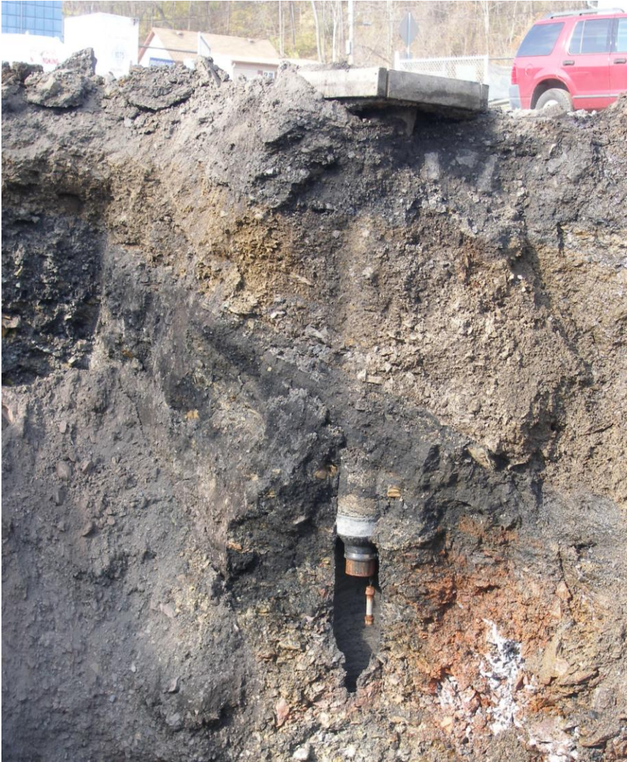
Figure 11 – iButton Drill-hole Installation Exposed by Excavation.
