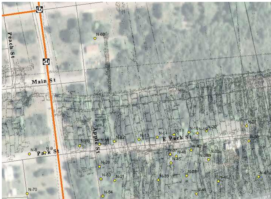
Figure 1 - Centralia Air Photo with Folio Mine Map and Drill-holes.
