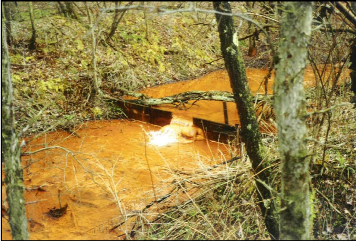
FIGURE 3 – Photograph of the mine drainage discharge from the abandoned North Penn Coal Company’s Snow Hill Mine showing the flow monitoring weir
