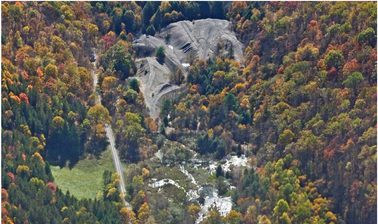
Figure 23. Refuse pile cast directly into stream valley near the headwaters of Mill Run in Fox Township, Elk County.
