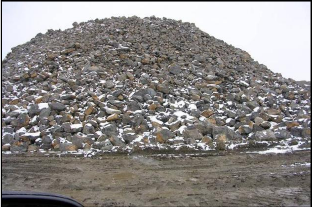
Figure 13 – Fall 2007 aerial view of remining operation on PA 1934 (above) and stockpile of limestone available for alkaline addition on PA 1934 site (below)
