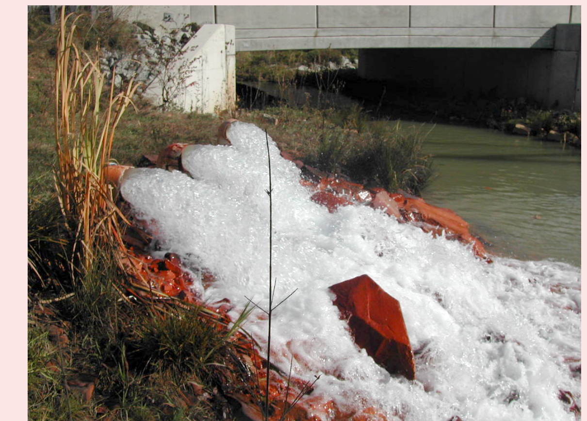
PA2530, Westmoreland County Measured Flow: 7,500 gallons per minute pH: 6.0, Total Iron 33.8 mg/l
