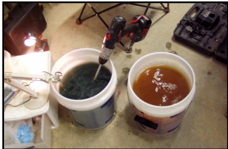
Figure Brandycamp-6. Comparison of hydrated lime dose tests during Brandycamp aeration study with AMD inlet on left and aerated AMD on right.
