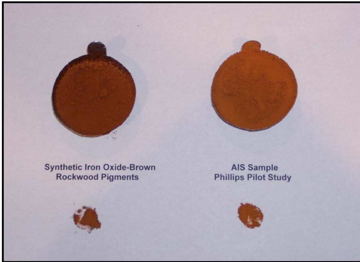
Figure FINAL-7. Comparison of a Synthetic Iron Oxide Pigment to an AIS Treatment Produced Iron Oxide.
