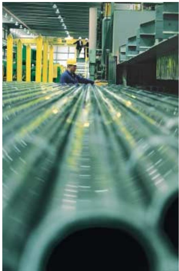
Pat Smith, Sharon Tube, checks tubes released on the drawbench for cooling, after entering the annealing furnace.
