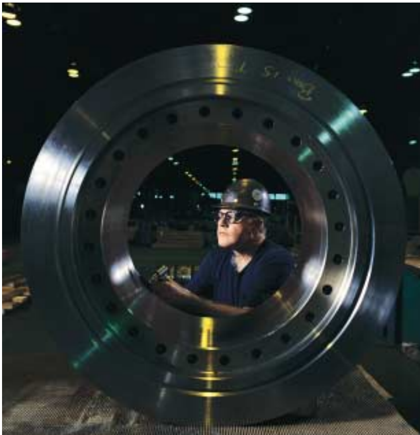
William Urbasic, Johnstown Corporation, finishes a sleeve used to roll steel. Steel rolling sleeves are among the products manufactured at the Johnstown Corporation.
