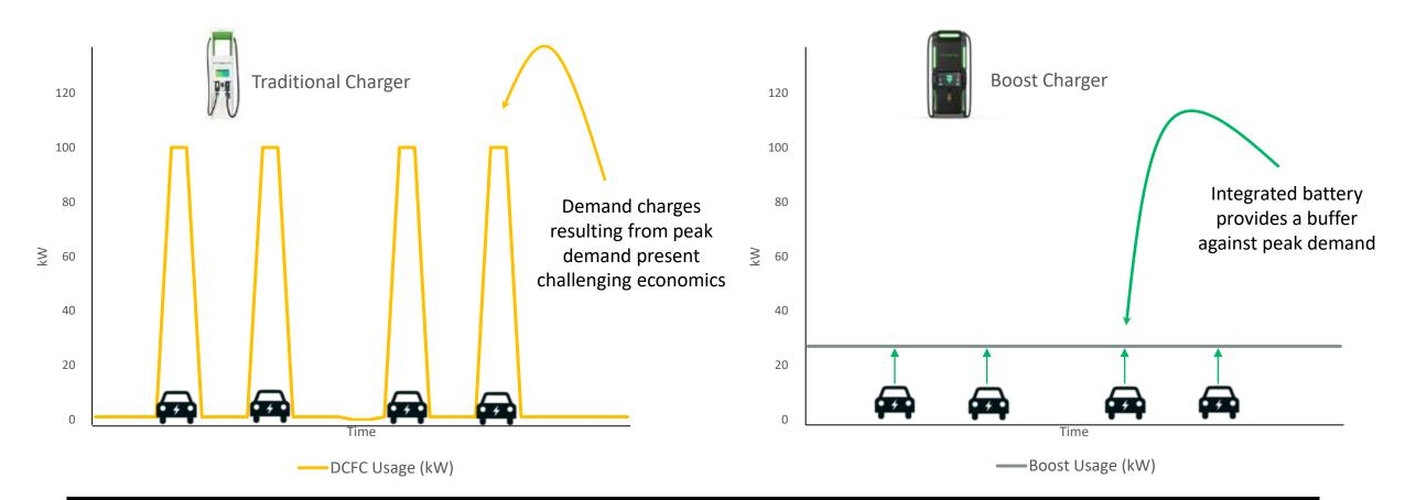
Integrated batteries reduce demand charges and can respond to TOU or other energy pricing mechanisms
