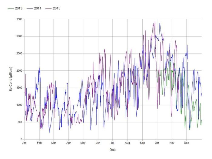
Figure 4. Continuous specific conductance from October 1, 2013 to November 15, 2015.
