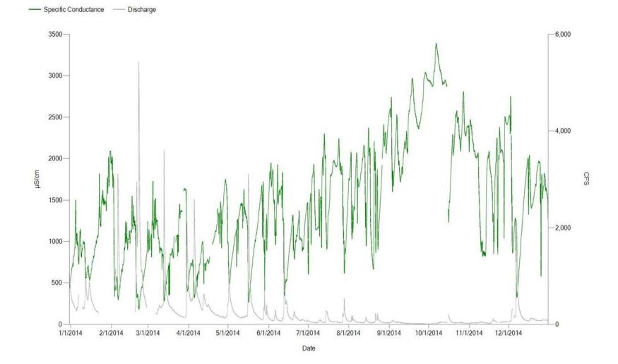
Figure 5. Continuous specific conductance from January 1, 2014 to December 31, 2014 illustrating depressed readings in response to elevated discharge events.
