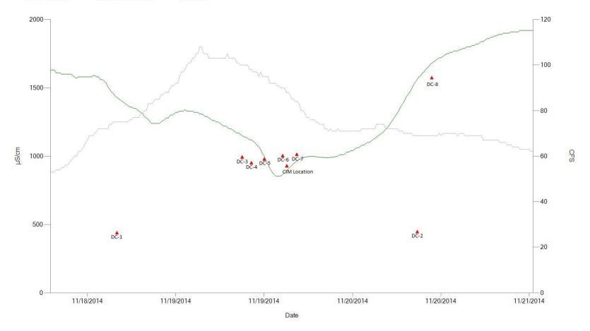
Figure 10. Specific conductance CIM data overlayed by discrete water quality readings taken during the stream assessment field data collection from November 18 to November 20, 2014.
